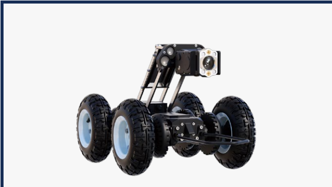
PIPELINE INSPECTION ROBOT
